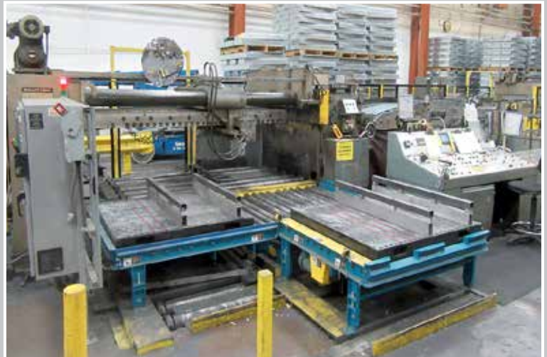
CINCINNATI Forte Blanking Line
