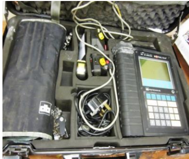
DB Pruftechnik AG Rotalign smart precision alignment unit
