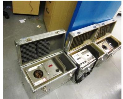
Haven Automation Tempcal 300 calibrators
