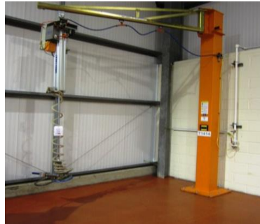
Palamatic handling system jib crane and suction lift
