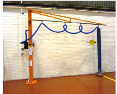
Palamatic handling system jib crane and suction lift
