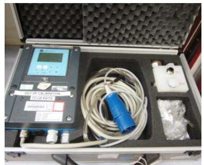
Endress Hauser Mycom 152 Concal conductivity calibration set
