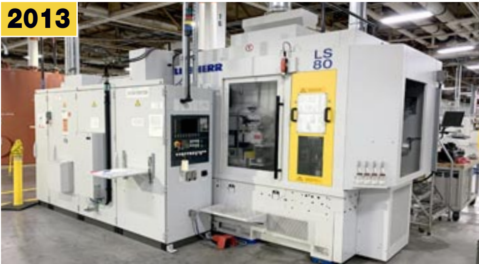
LIEBHERR LS-80 CNC Gear Shaper
