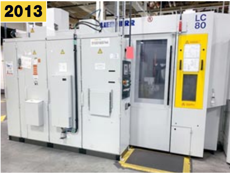
LIEBHERR LC-80 CNC Gear Hobber
