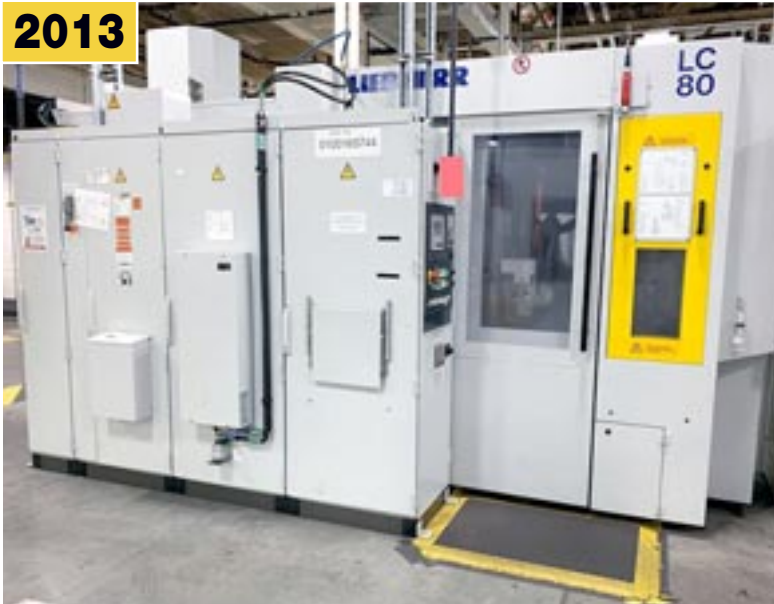
LIEBHERR LC-80 CNC Gear Hobber
