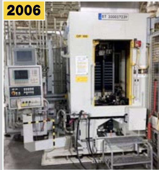
FORST TECHNOLOGIES CNC Broaching Machine
