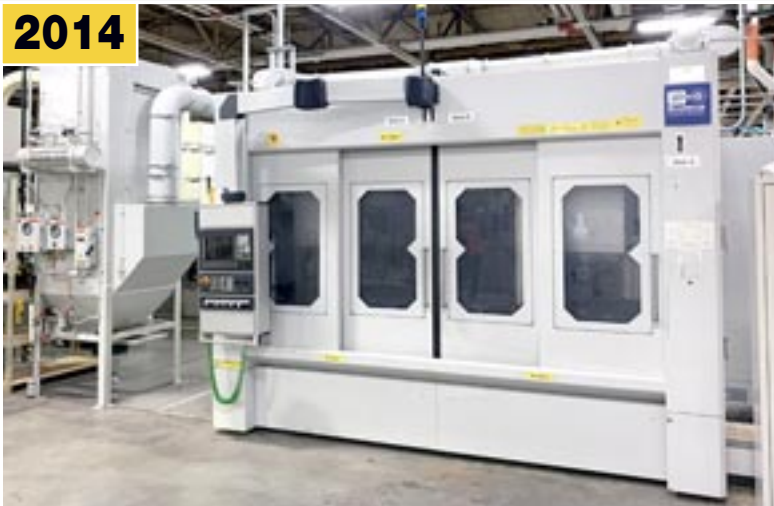
BUDERUS CNC 235 Vertical Hard Turning Machine
