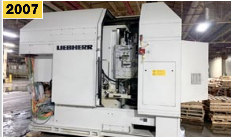
LIEBHERR LFS-220 CNC Gear Shaper
