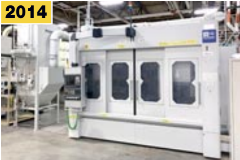
BUDERUS CNC 235 Vertical Hard Turning Machine
