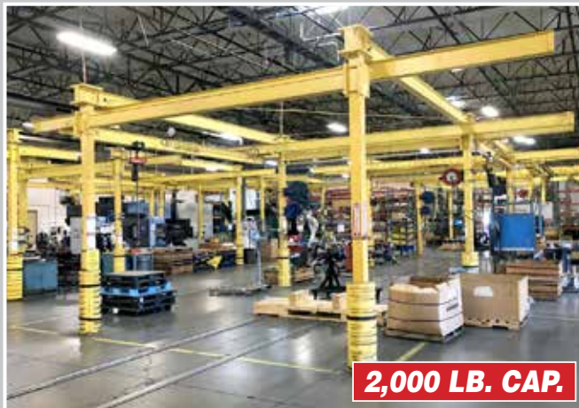
Freestanding Overhead Bridge Cranes
