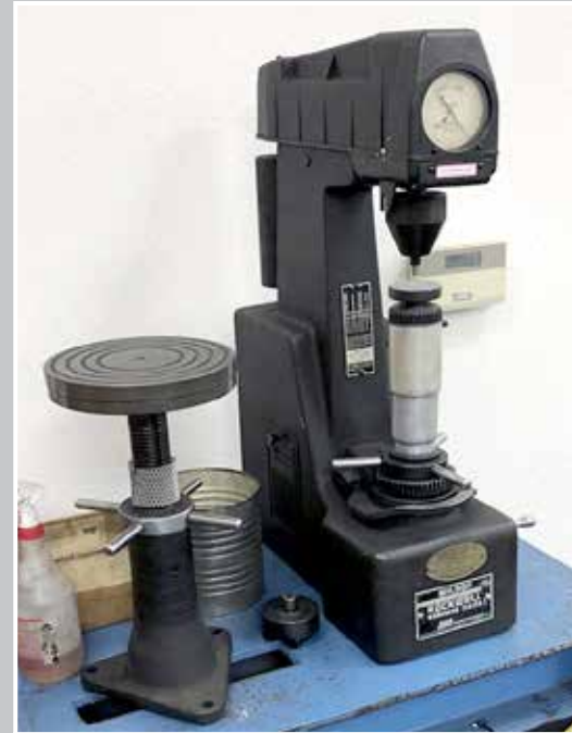
WILSON ROCKWELL 4JR Hardness Tester
