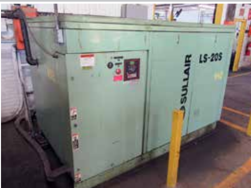
SULLAIR LS-20S-150 L AC Air Compressor
