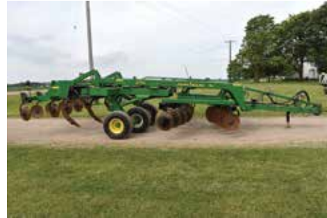
*** John Deere 2700 Ripper 5 Shank, Double Disc Front, Rear Levelers, Hydraulic Adjust Front Disc & Rear Levelers, SN: X001875
