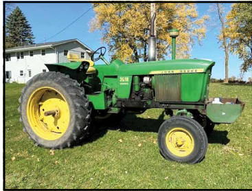
John Deere 3010, Diesel, WF, Single HYD, 3 PT, Missing Top Link, PTO, Fenders, Rock Box, Fenders, 13.6-36s, 261 Hours Showing (2) Leyland 384 Tractors For Parts Or Repair 18.4-38 Duals
